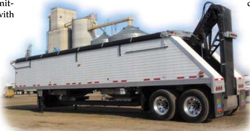
Our new Timpete trailer serves a dual purpose as a fertilizer conveyor or as a conventional hopper, depending on the season.
