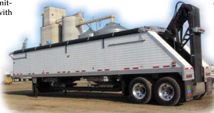
Our new Timppte trailer serves a dual purpose as a fertilizer conveyor or as a conventional hopper, depending on the season.
